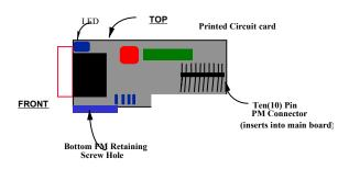
connector pins on the bottom of the PM card with the connector socket inside the unit. The pins are slightly angled to facilitate the installation. (Do NOT straighten the pins before insertion!!)
